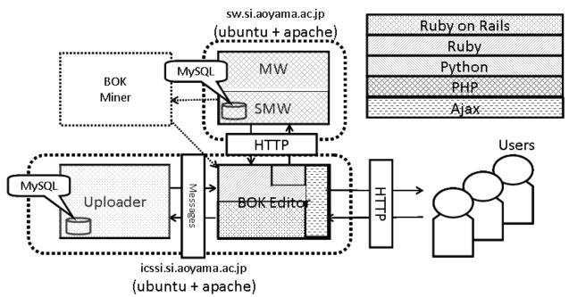
Figure 6. Details of BOK Constructor implementation.
