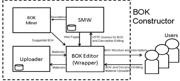
Figure 5. An overview of the BOK Constructor.
