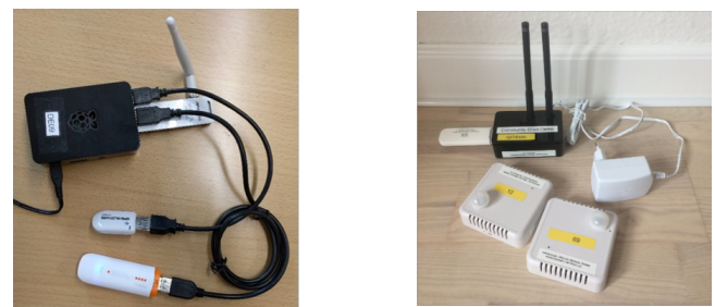
Figure 6: RaspberryPi and Environmental Sensors
